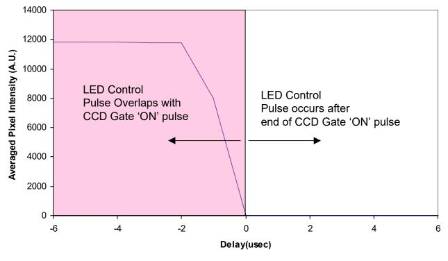
At 0 nsec delay The falling edge of the Gate Pulse coincides with the rising edge of the LED control pulse. However various delays within different system components may result in an additional relative delay of +/- 100nsecs.
